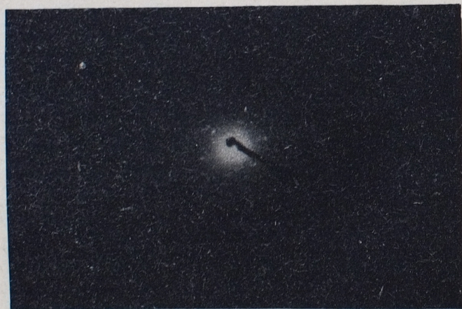
Phot. 2. Electron diffraction pattern illustrating the effects of the transformation of monoclinic [\text{Ca,Fe,Th}[\text{PO}_4]_2] /monazite group/ into hexagonal /rabdophane group/ [\text{Ca,Fe,Th}[\text{PO}_4]_2 \cdot \text{H}_2\text{O}] . Basal streaking and partly disordered spot pattern is related to monoclinic monazite pattern with spots belonging to 0\bar{1}1 zone axis chiefly. Streaking is probably caused by replacement of the monoclinic phase by a hexagonal one, developing parallel to \bar{1}11 /parting plane/. Pairs of spots with interplanar distances related to hexagonal rabdophane group are scattered amidst the monoclinic pattern
