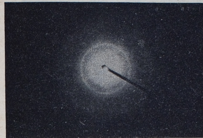
Phot. 3. Electron diffraction pattern illustrating the effects of transformation of hexagonal [\text{Ca,Fe,Th}[\text{PO}_4]_2 \cdot \text{H}_2\text{O}] /scattered pairs of spots/ into orthorhombic ultrafine-grained [\text{Ca,Fe}_{1-x}\text{Th}_{1-x}\text{RE}_{2x}[\text{PO}_4]_2 \cdot 2\text{H}_2\text{O}] related to ningyoite group /ring pattern/
